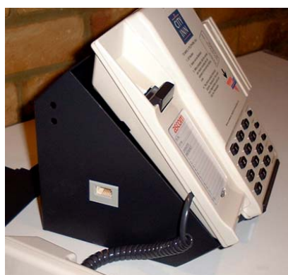
Phone drops into place in the housing. A modem socket is provided in the side panel.
